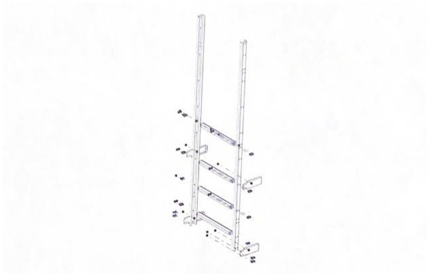
Figure 20 – Top Ladder Assembly
